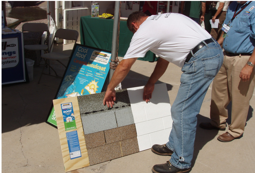
Our Roof Heat Test Prop at the 2007 Scottsdale (Arizona) Green Building Expo - October 2007. 15/32" Plywood with three different colors of asphalt shingles nailed on. The right side of the asphalt shingles is coated with 1 coat of Ceramic InsulSeal (primer) and 2 coats of Ceramic InsulCoat Roof (finish product).
